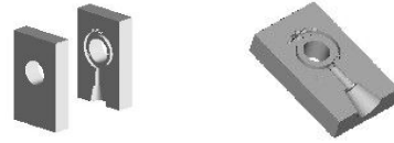
Fig.8. Ring molds created using Unigraphics (Left) and MAGIC (Right).
