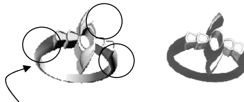
Fig.10. Ring models created by JewelCAD (left), and after fixed errors it still shows flipped triangles in black color (right).
