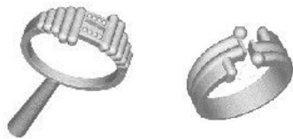
Fig.6. The second and the third examples of ring models created using JewelCAD and Unigraphics.
