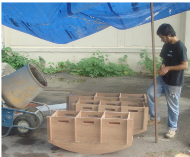
Fig. 9: Rocking mechanism for curing blocks.
