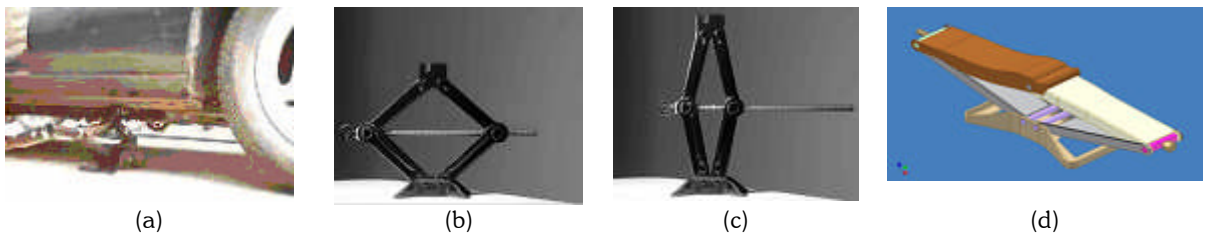
Fig. 3: Automobile jack example: (a) lifting location; (b) lowered position; (c) raised position; (d) CAD model.
