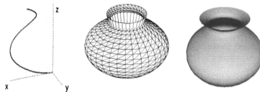
Fig. 2: Rotational Sweep: A profile curve, the surface of revolution, the shaded image [13].
